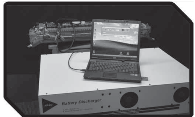
Figure 5. Hybrid battery module power test connections
